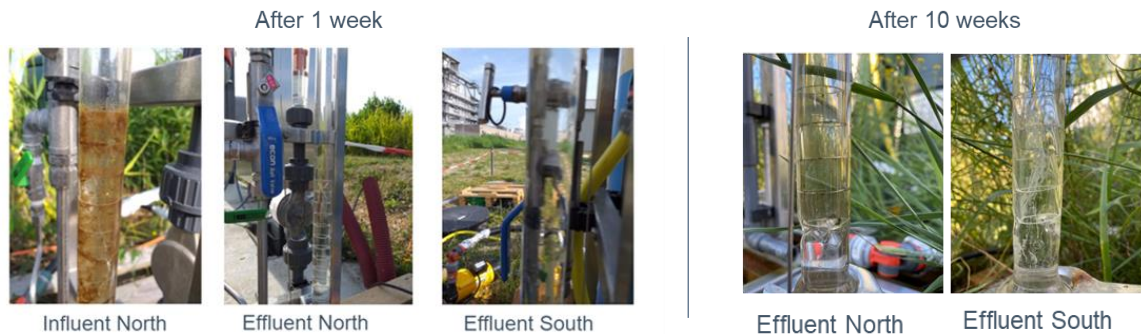
Figure 8. Biofilm monitor with wetlands North and South in series – visual results
