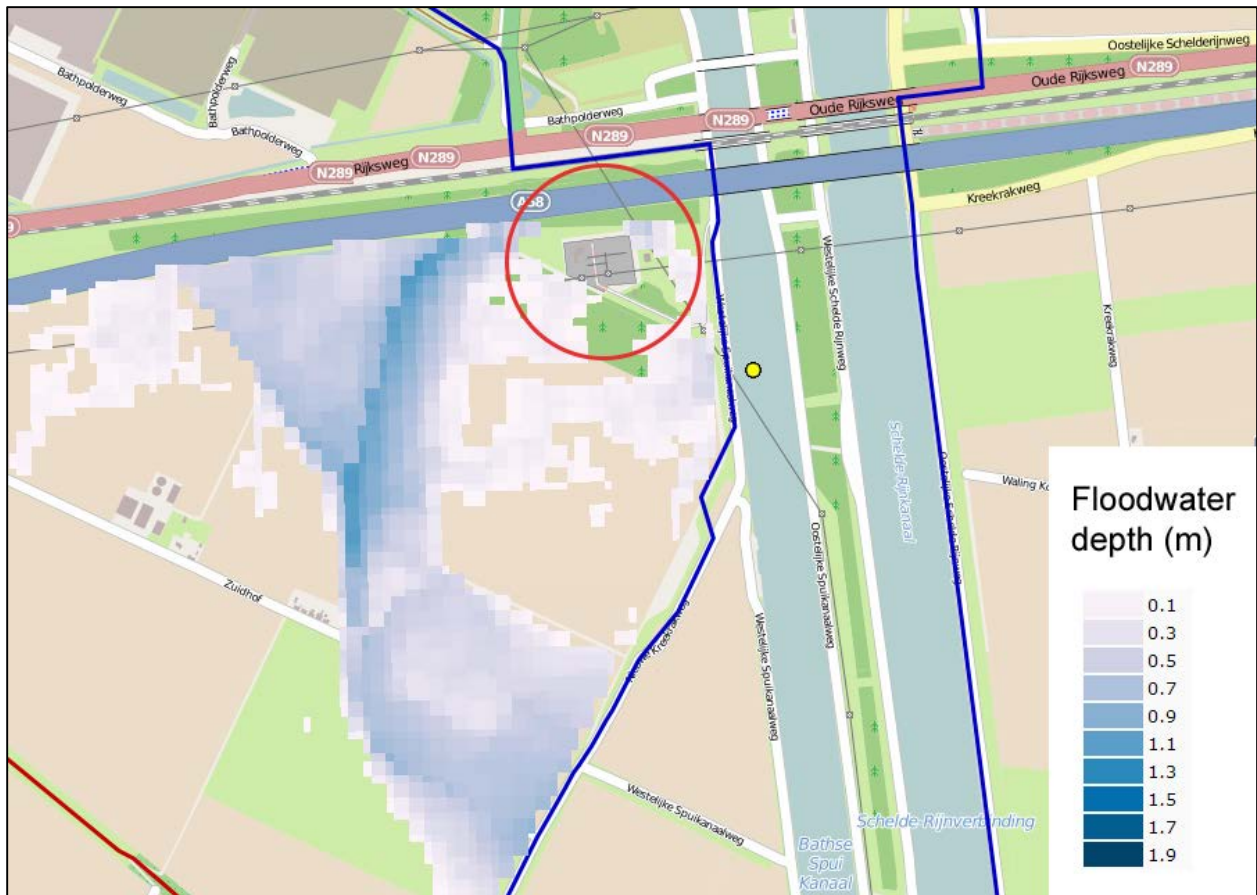
Figure 22. Close-up on the electrical sub-station 26. Generated from (Lizard Flooding, 2012) on July 18, 2014.
